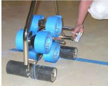
Position your chalk line under the right-rear wheel and continue under the right-front wheel. This will firmly anchor the chalk line and ensures an accurate guide line is produced.
