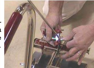
Loosen both thumb screws on the off-set pointer attachment. Slide it down onto the main pointer and tighten the thumb screw to secure it into position.
