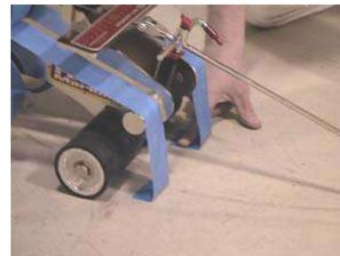
Pull the tape over the tape guide and stick it to the floor directly in front of the front wheels.
